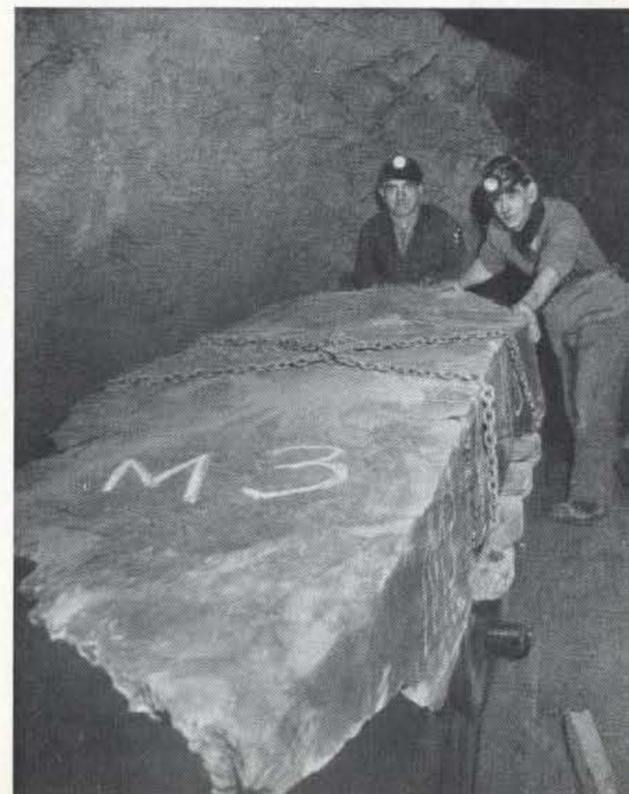
The trolley carrying the M3 block is pushed along the railway track through a short tunnel to the foot of the first upward haulage incline.
