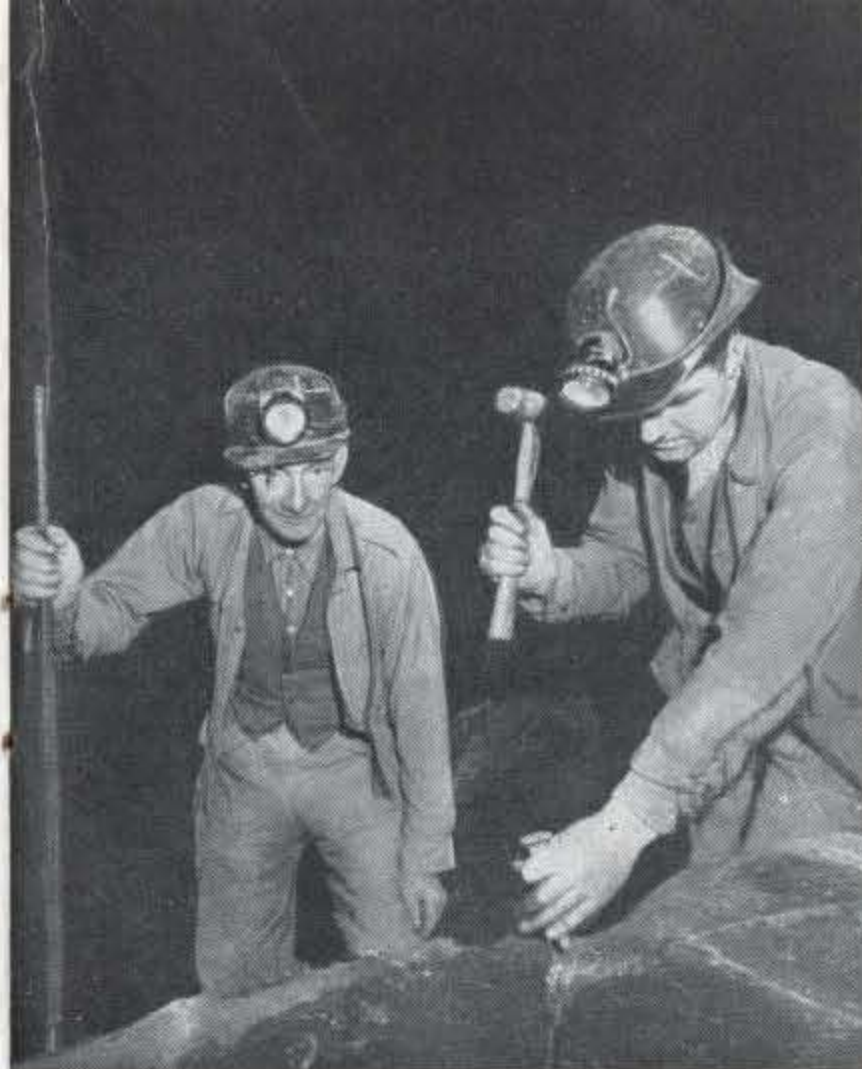
A massive block of slate, weighing about ten tons, is reduced by splitting it across the vein.
