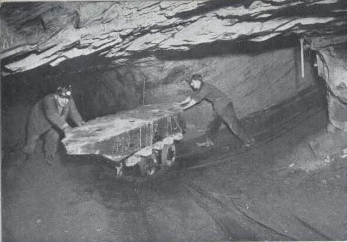
At the junction, the block is swung round on a turntable preparatory to hooking on to the power-drawn cable for haulage up the MK. incline
