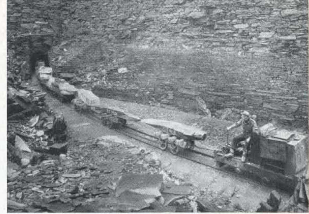
Exposed to daylight after millions of years the block emerges from the mine in a train of trolleys.
