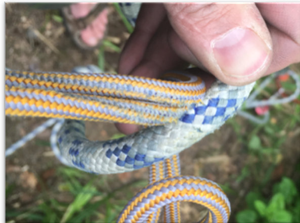
Figure 10. Prusik cord melted onto a rope. Photo by Gethin Thomas
