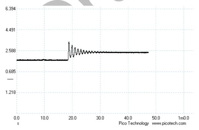
/Users/gethinthomas/Dropbox/LOMLA/Tyrolean Rigging/HeaveHo.doc Created on 13/12/2016 13:21:00 www.train4underground.co.uk Page 3 of 8 Prior to the drop the rope was tensioned by 2 of us to 1.718kN. The peak impact was 3.423kN with the load stabilising at 2.455kN.
