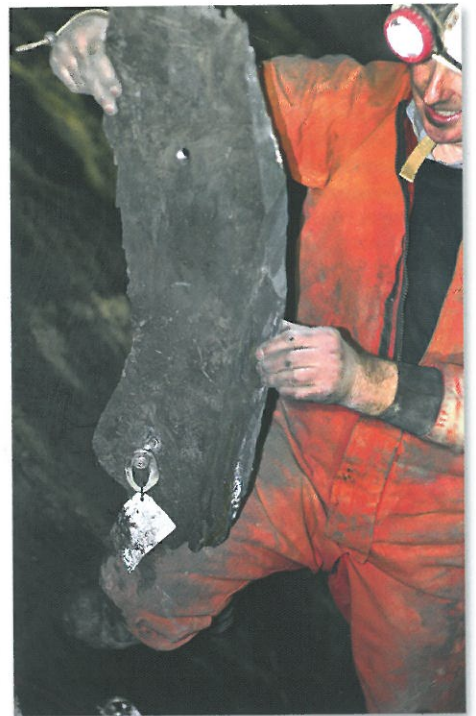
A flake of slate loosened by the first anchor extracted (leaving a hole) and released from the rock face by a second anchor (still attached) Photos: Gethin Thomas
